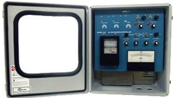
For certain applications it may be necessary to add both acid and caustic. Optional set points permit high and low addition at different values leaving a middle range where neither is added. In other applications the second set point may add neutralizer at a higher rate than the first one, Similar to proportional control.
